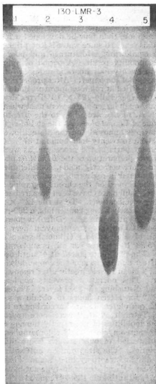
Fig. 1.—Paper chromatography of preparations using 2% p -toluenesulfonic acid monohydrate in water saturated n -butanol as the developing solvent at room temperature; development period 24 hours: zone 1, 0.4 unit mannosidostreptomycin; zone 2, 0.2 unit of streptomycin A; zone 3, 0.4 unit of dihydrostreptomycin A; zone 4, 0.4 unit of neomycin A, and zone 5, 0.4 unit each of streptomycin A and mannosidostreptomycin. All antibiotics are sulfates. A one inch square of paper is shown on each chromatogram.
